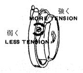
糸の張力は、小さいほど良い。 Tension on threads should be as light as possible, while still sufficient to set stitch correctly in material. 上糸張力の調整の仕方 NEEDLE THREAD
