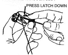
THREAD PULLED DOWN THROUGH SLOT
