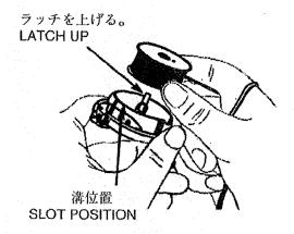
Replacing Bobbin in Case
